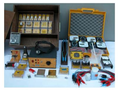
The kit is composed of a set of components and devices that allow a practical demonstration of the most important laws of electricity and electromagnetism.
