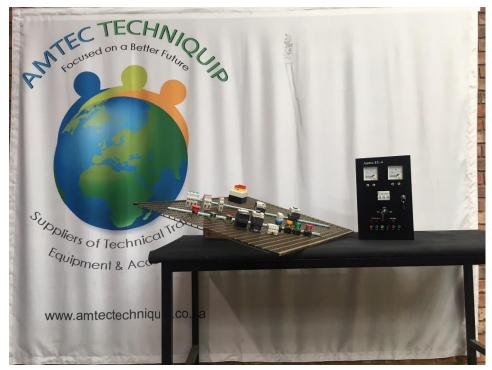
Set is comprised of a grid type frame and power supply unit mounted to a workstation.
