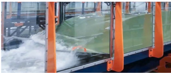
Braided river, accumulations of logs and flood sediment studied in an Armfield research flume
