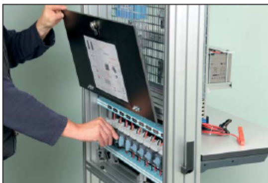
Flap for access to the switches
