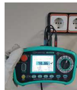
Loop test from a wall socket
