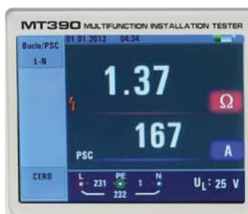
Dual line display with correct wiring indication
