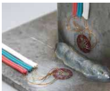
Weld bead (rosette strain gauge)
